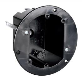
3 3/4-inch Round Old Work Box with Swing brackets for mounting that adjust from 1 1/4-inch down to 1/8-in. Four Auto/Clamps, Includes Device mounting holes. 50 pack.
