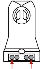
Connect wires directly to these terminals
