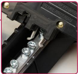
Our innovative split neutrals save you time and wire by allowing Plug-on Neutral circuit breakers to connect directly to the neutral bar without a pigtail. Coupled with the innovative design, our neutral bars are now fully-distributed, accepting Plug-on Neutral breakers on any space.
