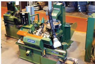
A Modern Up to Date Roll Threading Machine at our Affiliate, Avanti Screw.
